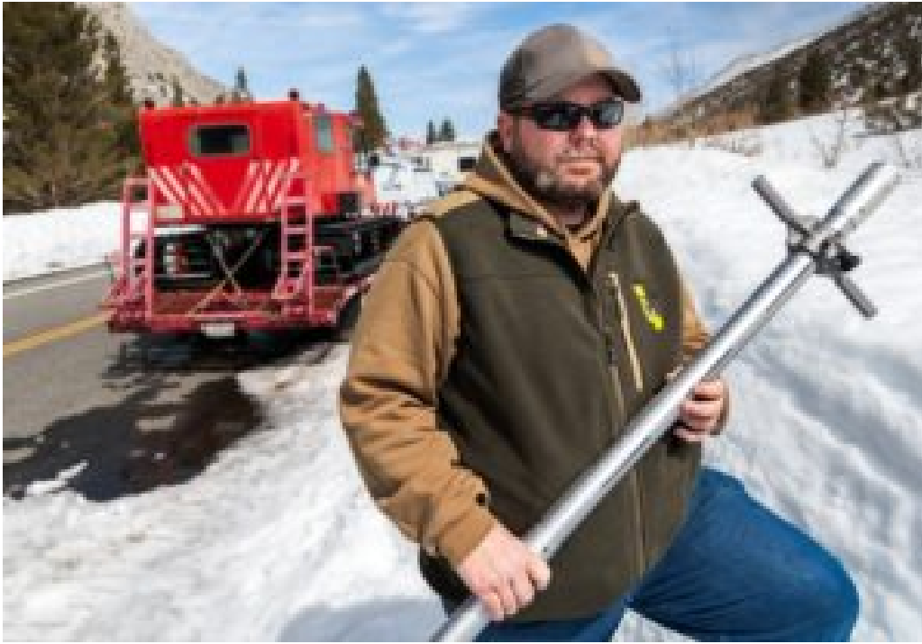
Senior Hydrographer Bruce Peterson holds aluminum tube used for taking snow core samples.
